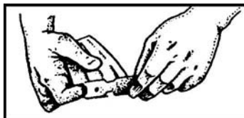
Figure 071-311-2025-41. Removing the base of the magazine
