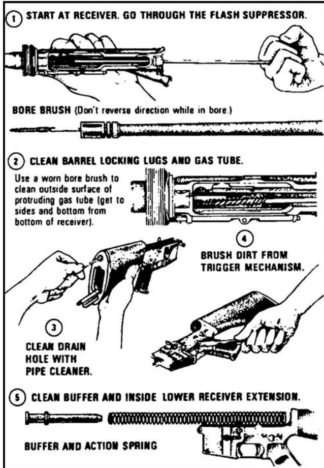
Figure 071-311-2025-21. Cleaning the receivers
