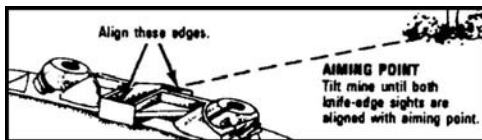
Figure 071-325-4425-8. Aiming knife-edge sight (continued)
