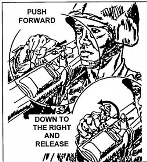
Figure 071-054-0001-5. Cocking the launcher
